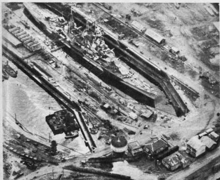
Flying over Brest Harbor , an RAF Coastal Command pilot took this reconnaissance picture of a Hipper Class cruiser at 500 ft. Sloping cinder screen and bulbous directors are typically German features.
